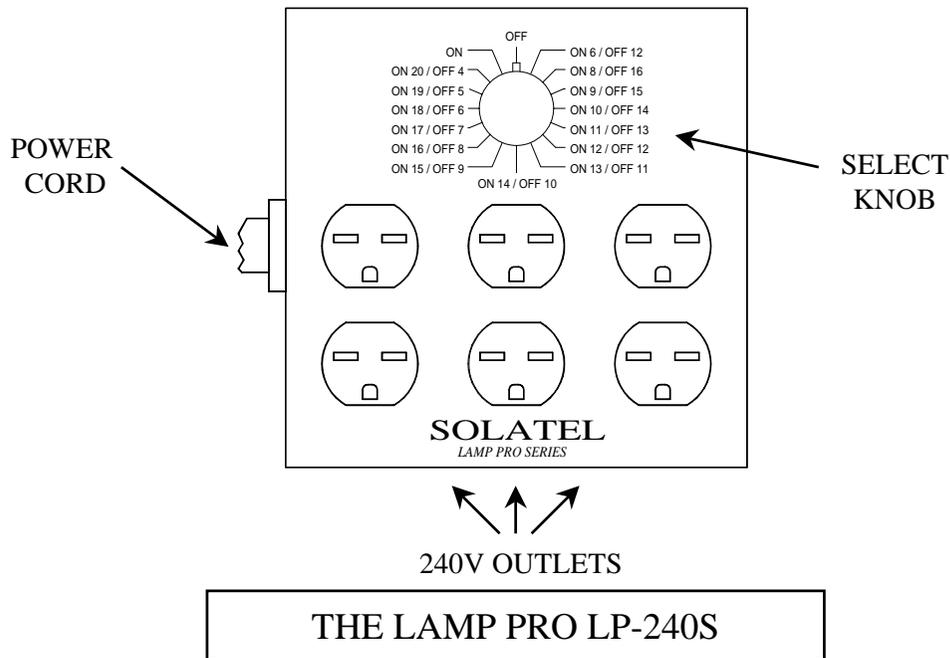
The Solatel LP-240S is a member of the Lamp Pro series of timers. It is easy to use with a single Select knob that clicks to any of 16 time settings. Settings include an accelerated 18 hour day cycle running ON 6 HOURS / OFF 12 HOURS. Thirteen normal 24 hour day settings cover ON 8 / OFF 16 to ON 20 / OFF 4 in one hour increments for growing both short day and long day plants. Also included are continuously ON and OFF settings.
