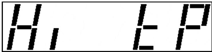
(alternates) between time and sensor readings. The overtemp display only occurs when the Select Knob points to RUN. All other positions are normal. It is blanked by Display Blanking At Night mode when the lamp would normally be off. Any fault, including Clock Fault, Setting Fault, Flood Fault or Panic Fault causes the display to flash. It still shows the alternating message and temperature but they are flashed. When the fault ends, overtemp display continues if still valid.
